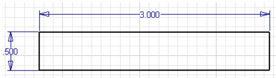
Figure 3.4.10: Dimensioned Sketch of Support Member
